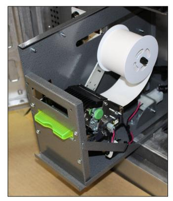
After following the paper unload procedure, slide a new paper roll onto the printer shaft with a paper in the orientation as shown below.
