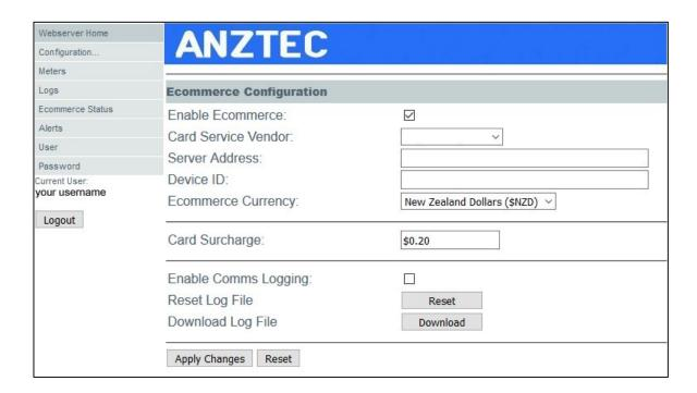
To enable ecommerce communications logging, make sure the Comms Logging box is checked.
