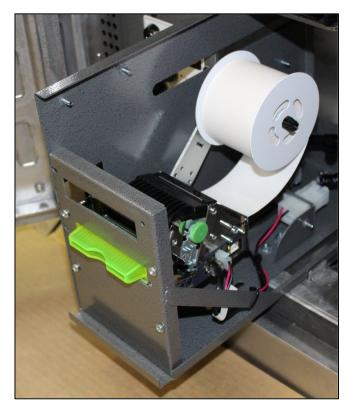
Press the paper retainer back onto the shaft.
