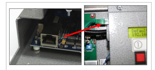
QW-5960P network connector is hidden under the edge of the Network Status Display cover.
