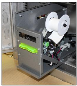
Align the slot on the paper retainer with one of the four retaining fins on the paper roll shaft.
