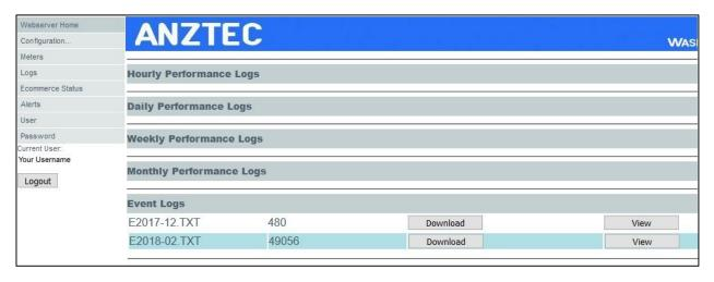
To view the log without downloading press the View button and use the previous and next page button to scroll through the log.
