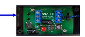
Connect 24VAC wash start signal lines from your car wash into connections 1 and 3 on connector S1 in the Wash Open Interface Unit
