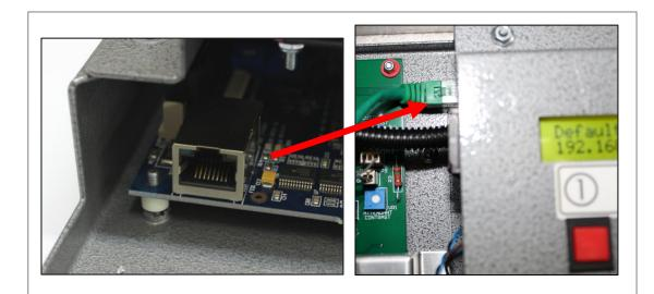
QW-5962N network connector is hidden under the edge of the Network Status Display cover.
