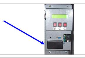
Feed the 24VAC wash start signal lines from your car wash through the hole in the Wash Open Interface Unit
