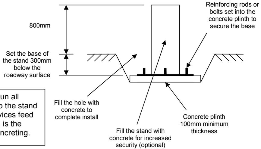
**Note:** Make sure you have run all services through the plinth to the stand and into the rectangular services feed cutout area. Check the base is the correct orientation before concreting.
