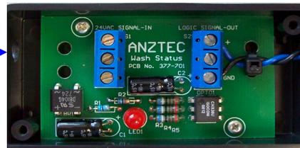
Connect 24VAC wash start signal lines from your car wash into connections 1 and 3 on connector S1 in the Wash Open Interface Unit
