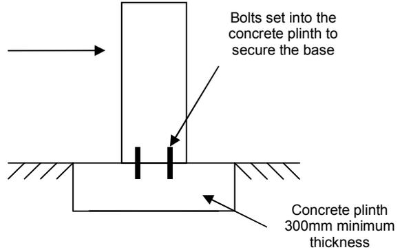
**Note:** Make sure you have run all services through the plinth to the stand and into the circular services feed cutout area. Check the base is the correct orientation before concreting.
