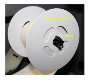
Press the fins together and pull off the paper retainer.
