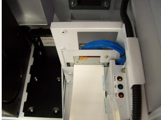
5. Push the printer back into its normal operating position. This enables the paper to feed out through the receipt slot in the front panel.
