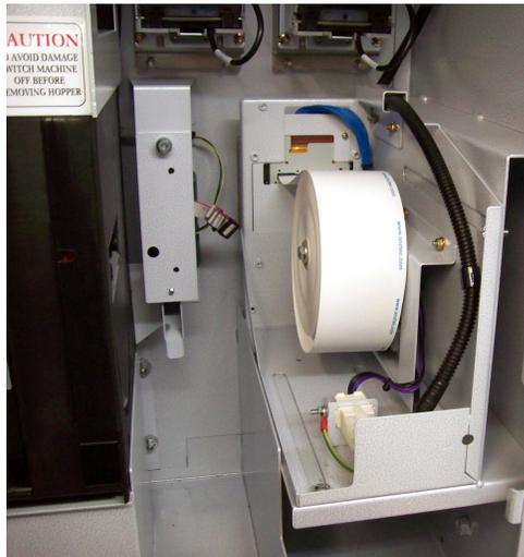
6. Turn on the machine power the paper should automatically feed into the printer.
